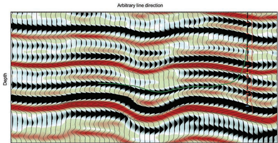
Figure 12. Final PSDM image and well trajectory of recently completed well. The PSDM was performed as part of the study presented in this publication. As confirmed by well data, the PSDM reveals the correct positioning of the producing shale layer. During drilling of the well shown here, the well went out of zone and then was directed back to the producing zone. If accurate PSDM data is generated prior to drilling campaign, drilling out of zone can be minimized.
