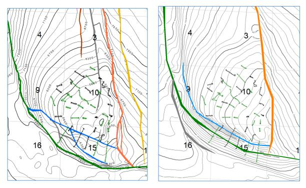
*Figure 1. Beaver Creek Field structure based on PSTM data (Left) and PSDM data (Right). Only wells utilized in the CO2 flood are posted.*
